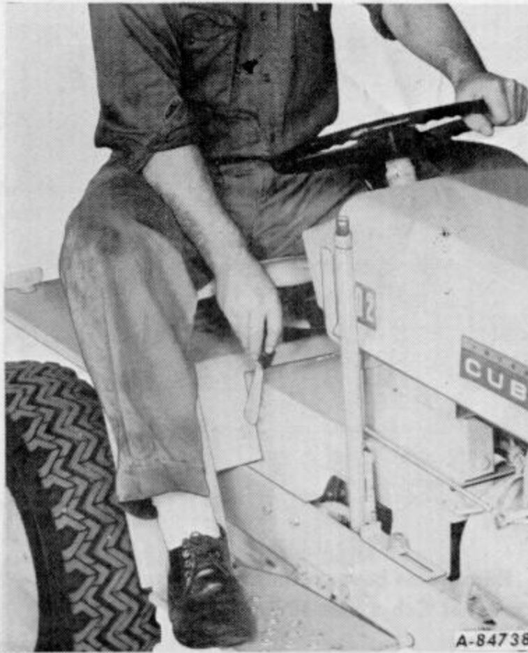
Illustr. 19 Operating the Power Take-Off. (International Cub Cadet 102 and 122 Tractors).
